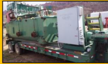
3200 Gallon Portable Mud Pit Equipped with Derrick Linear Shaker, 2- 3x4 Centrifugal pumps, mud hopper and pits jets, Electrical panel, Tandem axle trailer $31,500
