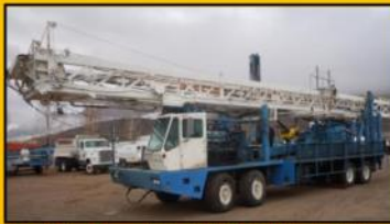
2000 Gefco Speedstar 150K P/B Detroit Series 60 (475 hp) 6 spd. Auto Trans., 58'x150,000 lb cap. Derrick, top-head drive w/47' travel/clearance. Excellent Condition! $435K
