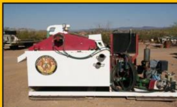
2006 Portable Mud System 750 gallon tank, Shale Shaker, Centrifugal pump and desanding, Cone and Lift pump. $35,000
