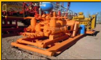
Ideal C250 7 1/4 x 15 Duplex Mud Pump P/B Detroit 8V-92 Diesel Eng., w/Elec. Starter, Radiator, Gauges, Twin Disc PTO, Master Skidded $29,500
