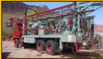
Gardner Denver 2000 Mntd. on CCC 4 axle, P/B Cumm. 400, Newer 58' Derrick, 54m Stacked DD, 5" x 8" pump, WEJ Air Comp., 10" retract Rotary Table. Excellent Condition! $345K
