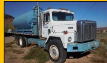
1982 Paystar International 5000 P/B Cummins 350 Eng., 9 spd trans., 100 Barrel Skid Mntd., Self Propelled Vacuum Tank $18,500
